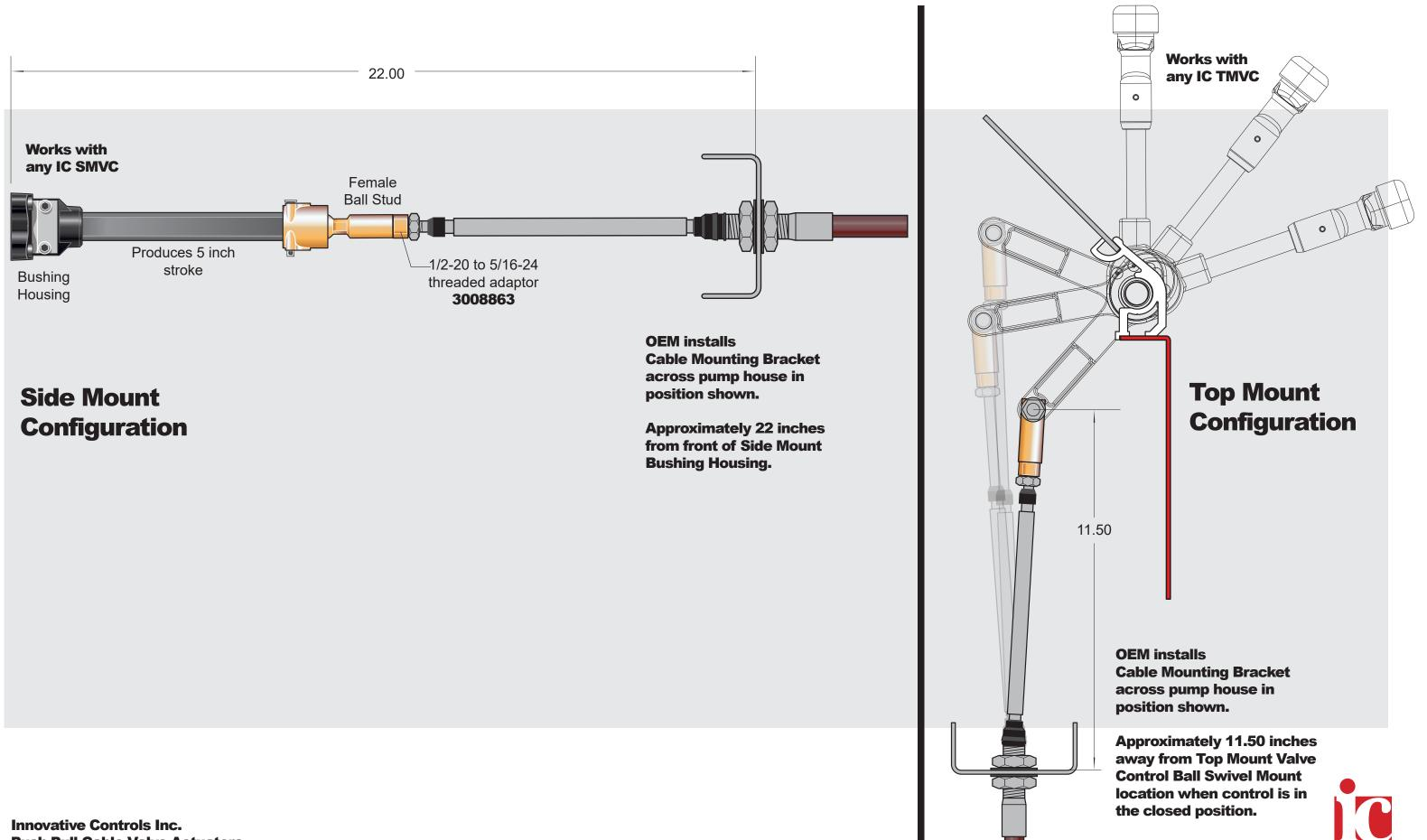
Push Pull Cable Valve Actuators Control-End Mounting Configurations
